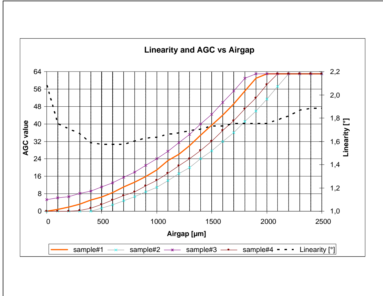
Figure 27. Typical Curves for Vertical Distance versus AGC Value on Several Untrimmed Samples
