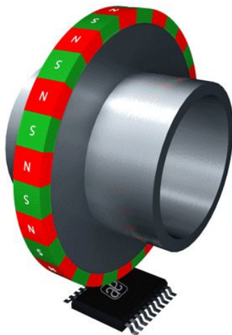
Fig. 5: Off-axis rotation angle measurement with multipole ring and radial mounting of the sensor
