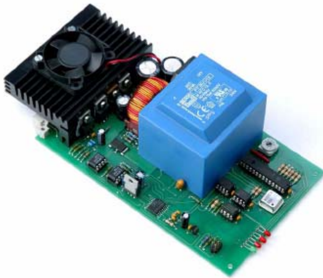
PCB-power supply with Ah-meter for drum electroplating
